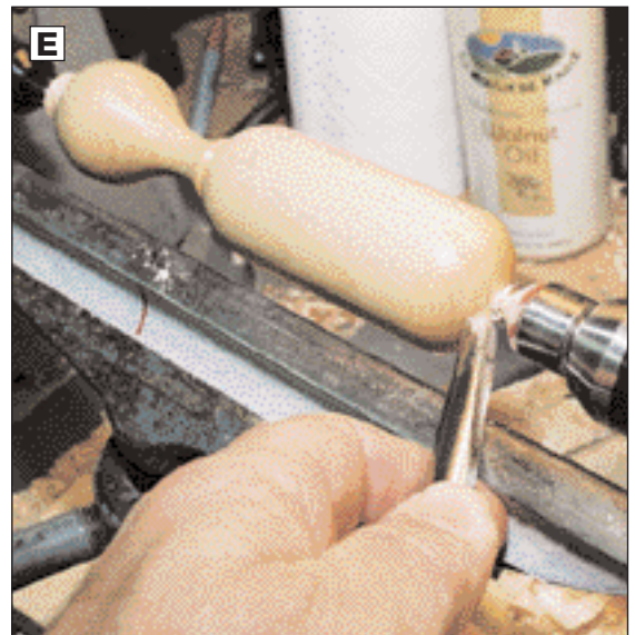
E With a 1/2" spindle gouge, part off the rattle end. A long fingernail grind guarantees success.
