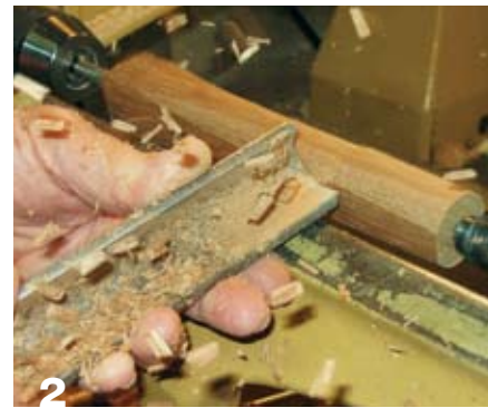
2 Use a spindle roughing gouge to turn the square workpiece into a cylinder.
