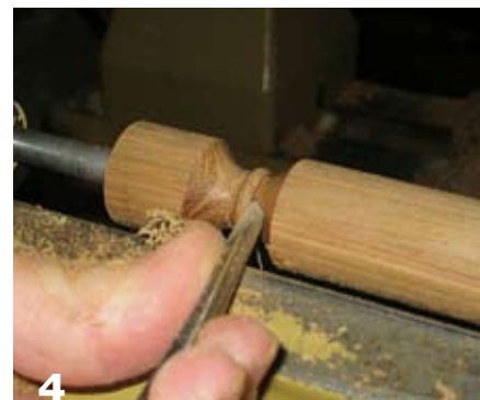
4 Complete most of the detail work with a \frac{3}{8} " or \frac{1}{2} " spindle gouge.
