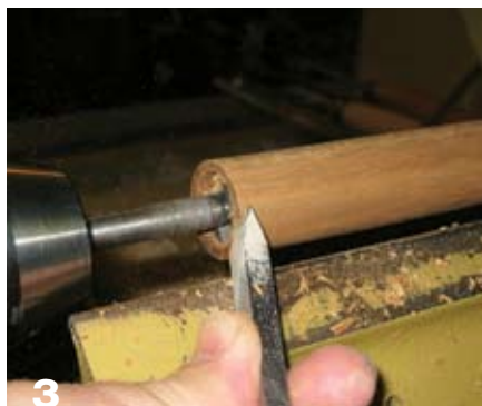
3 With a skew, make a peeling cut across the bristle end of the handle.
