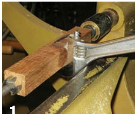
1 Use an adjustable wrench resting on the tool rest to hold the workpiece while drilling a socket in one end.
