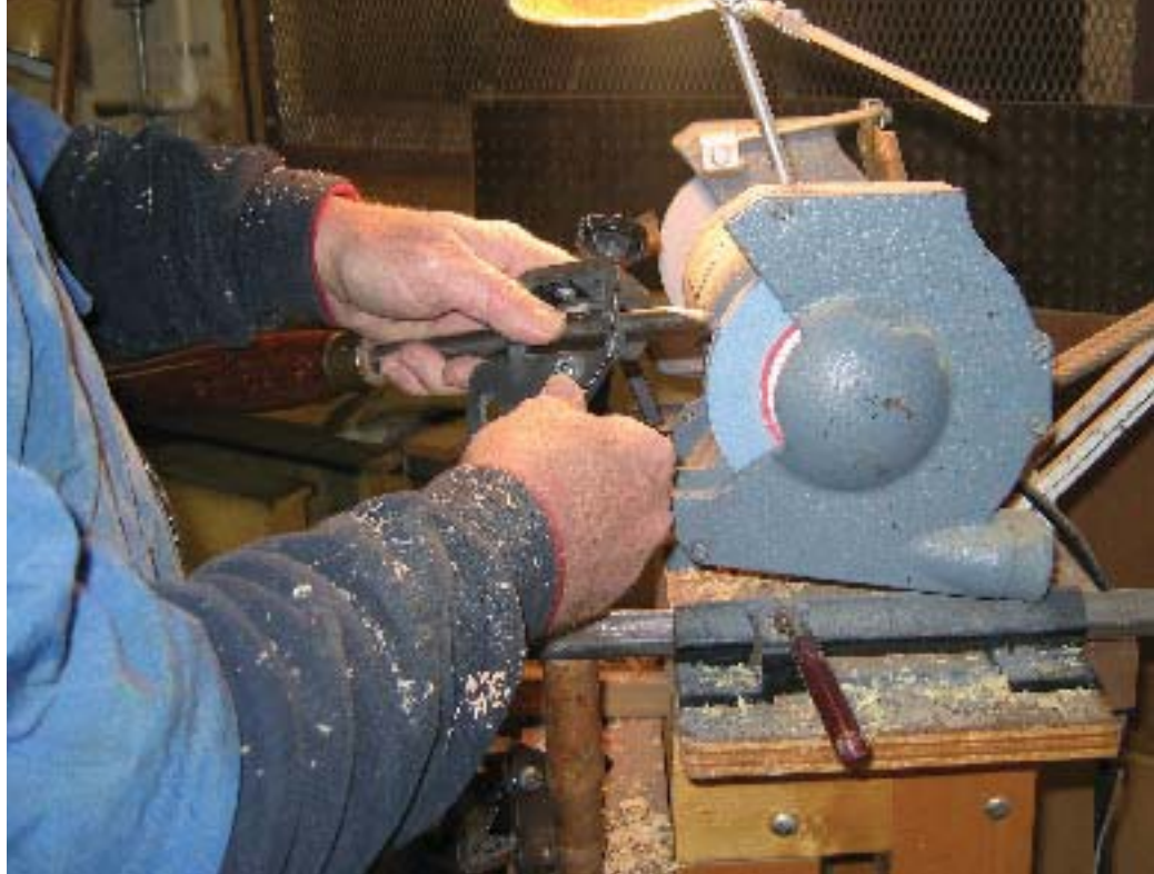
A grinding jig helps many new turners repeat the same bevel on a lathe tool.
