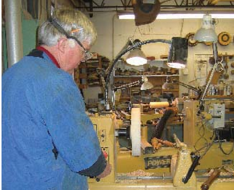
Here's a good habit to develop: Before you turn on your lathe, always stand to the left or right of the chuck.
