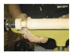
For additional support and better control of your spindle turning, wrap your index finger around the tool rest.
