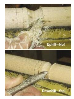
Always cut downhill, from large diameter to small diameter on spindles. Attempting to cut uphill on some woods will produce disastrous results—expect a lot of catches.
