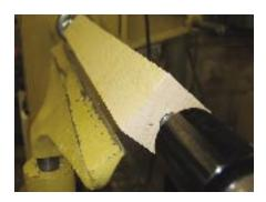
Adjust the height of the tool rest to match the tool you are using. You should cut above center for most lathe tools. If you switch from a thick tool (like a spindle roughing gouge) to a thinner tool (like a skew) you will need to raise the tool rest.
