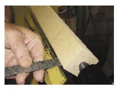
**Position the tool rest** parallel to the blank and as close as possible—1/4" is adequate clearance. Be sure to lock the tool rest to the support and the support to the lathe bed. Always rotate the workpiece by hand before turning on the machine. No matter how many times you have seen it done in demos, never move the tool rest with the machine running. Always move the tool rest closer after removing the corners from the blank—excessive overhang of the tool will cause chatter.
